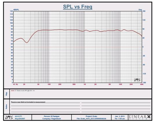
On axis SPL curve, 2.83V at 1m distance, 39Hz to 31kHz +/-3dB, 42Hz to 27kHz +/-2dB
