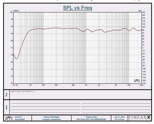
On axis SPL curve, 2.83V at 1m distance, 39Hz to 31kHz +/-3dB, 42Hz to 27kHz +/-2dB
